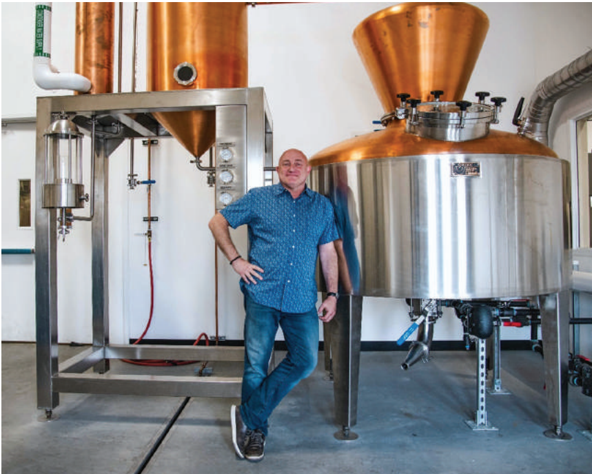
Golden Moon's Founder and Head Distiller Stephen Gould beside the 1000 litre SM still with an inverted cone head and custom expansion chamber beside the copper condenser
